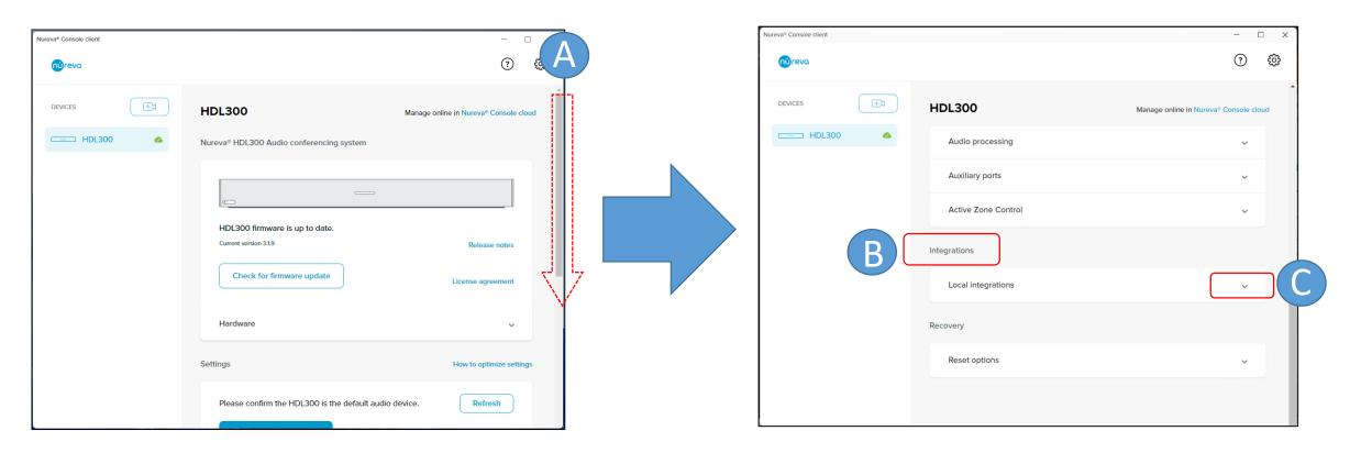
A: Drag the vertical scroll bar of the Console client downB: Scroll down until you see the 'Integrations' optionC: Click the down arrow of [Local integrations]
